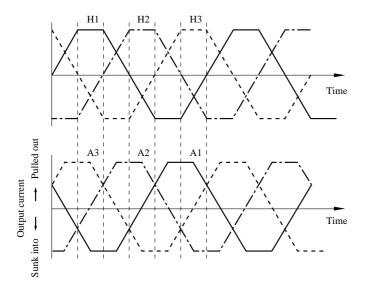
When EC > ECR, the pulling-out and sinking-into of the output current is just reversed from those shown in the above figure, and the motor rotation direction is reversed.
