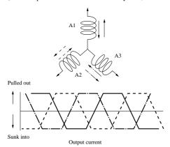
The AN8294S employs highly effective three-phase full-wave drive system, by which current is pulled out or sunk from/into each phase, A1, A2 and A3.
