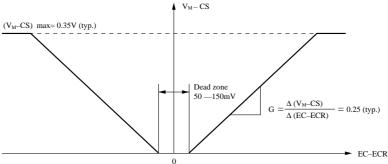
The G shown in the above figure and  $(V_M-CS)$  max. are almost stable, independent of current detection resistance (resistance between  $V_M$  and CS terminals),  $R_{CS}$ . For example, if  $R_{CS}=0.5\Omega$ ,
