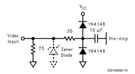
FIGURE 5. Recommended Video Input ESD Protection
