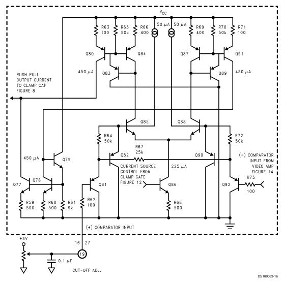
FIGURE 11. Simplified Schematic of LM1208 Clamp Comparator Circuit
