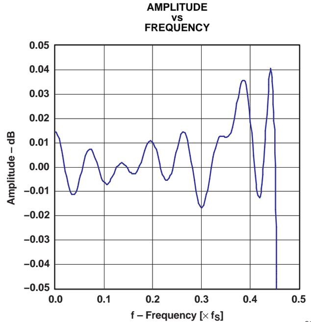
Figure 2. Pass-Band Ripple
