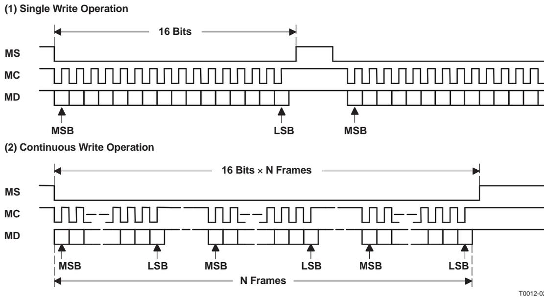
Figure 27. SPI Write Operation
