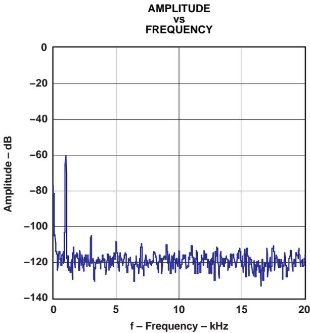
Figure 19. Output Spectrum (-60 dB, N = 8192)
