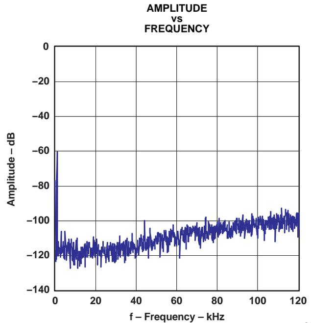
Figure 20. Output Spectrum (-60 dB, N = 8192)
