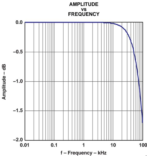
Figure 3. Pass-Band Characteristics
