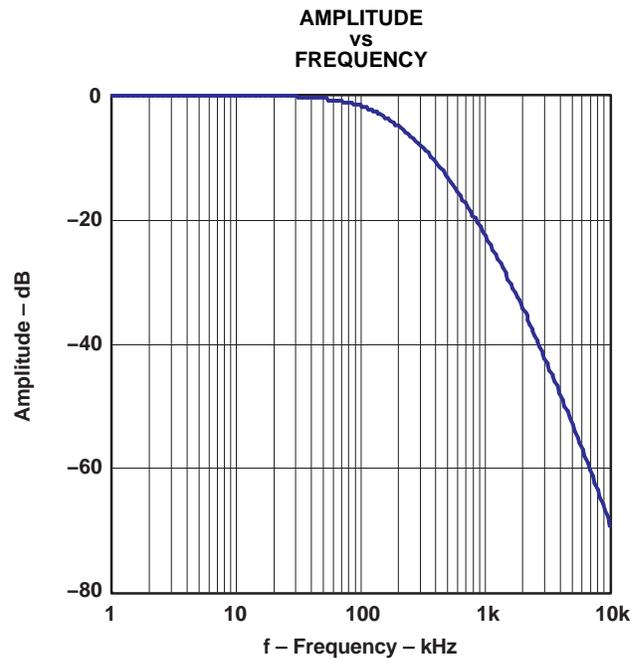
Figure 4. Stop-Band Characteristics
